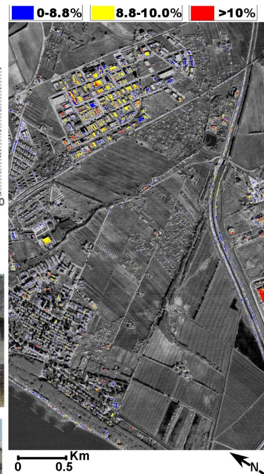
AC deterioration status map in the Follonica industrial area using MIVIS airborne data
